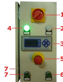
1. Main switch with the possibility to lock in position "0" (prevents from an use of the machine by unauthorized persons)
