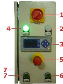
1. Main switch with the possibility to lock in position "0" (prevents from an use of the machine by unauthorized persons)
