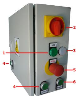
1. The green light "POWER" indicates a connection of the bale to power and that the main switch is turned ON
