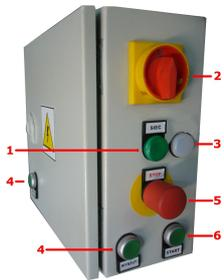
1. The green light "POWER" indicates a connection of the bale to power and that the main switch is turned ON
